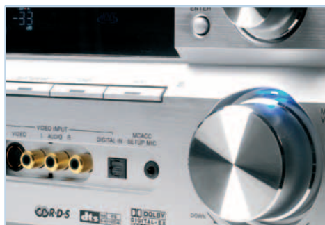
The front panel has an optical input as well as the regular AV ones
