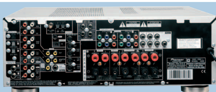
Options on the backside include 5.1 inputs for multi-channel music and the facility to bi-wire front speakers or use a second zone
